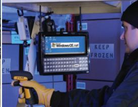
The VX6 is a half-screen Vehicle Mount Computer equipped with the Intel® XScale® processor and running Microsoft® Windows® CE .NET. Sealed against water and dust (IP66), resistant to shocks and vibrations, and supporting low temperature operation (-22° F / -30° C), the VX6 is the ideal tool for extreme warehousing operations, including cold stores.
