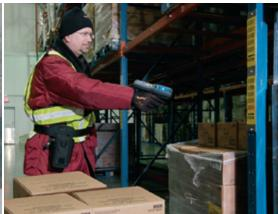
The MX7CS rugged handheld computer is built for your freezer and cold storage applications. Designed with low-temperature batteries, specialised heaters and conformal coating, the MX7CS unit adapts easily from the freezing temperatures of your storage areas to warmer staging and dock areas - even in the hot summer months. This smooth, condensation-free transition will allow your operators to increase productivity.
