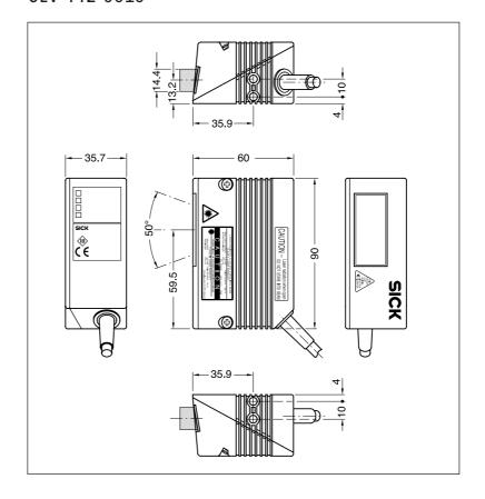
Line scanner with oscillating mirror CLV 440-6010
