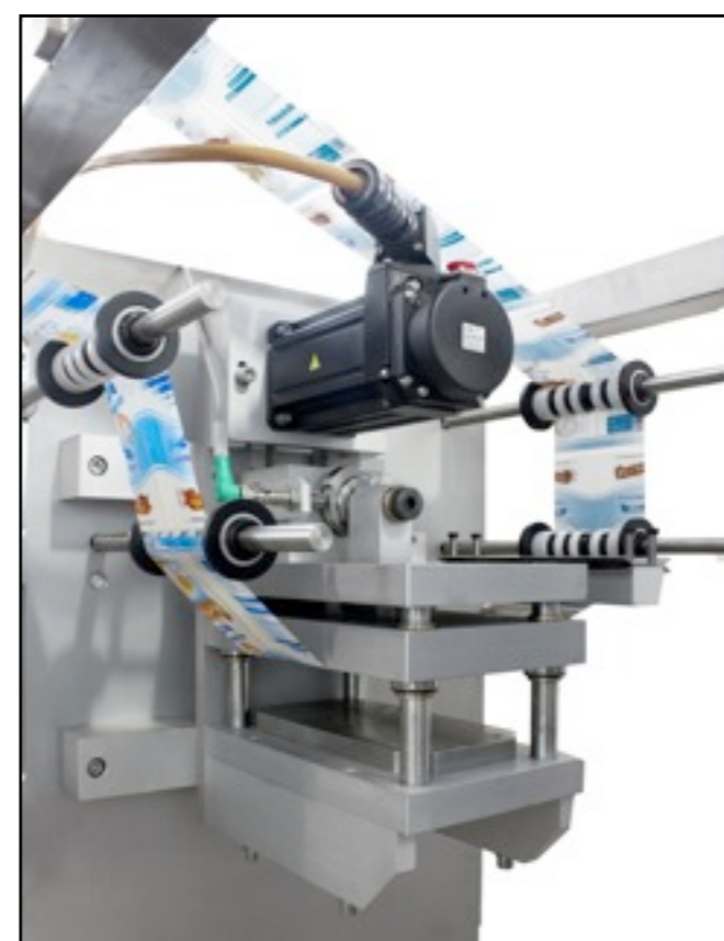
mechanical preperforator (up to 42,000 bph)
