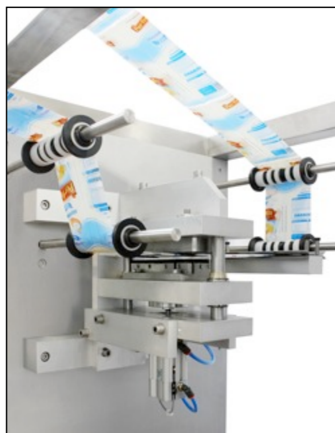
pneumatic preperforator (up to 15,000 bph)
