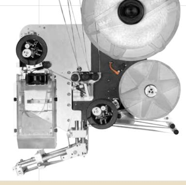
In the rewinder, the variable diameter mandrel facilitates removal of the silicon liner. The mandrel is usually expanded so that the operator does not have to carry out any operation and cannot forget to enable it The label reel housing employs a special polymer disk, hardened with fiberglass, to adequately support the heaviest reels even in the case of a labeler positioned horizontally
