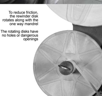
The reel securing plaque is transparent, light and takes up little space. Equipped with ergonomic handle, it can be quickly removed with a rotation of only 60°
